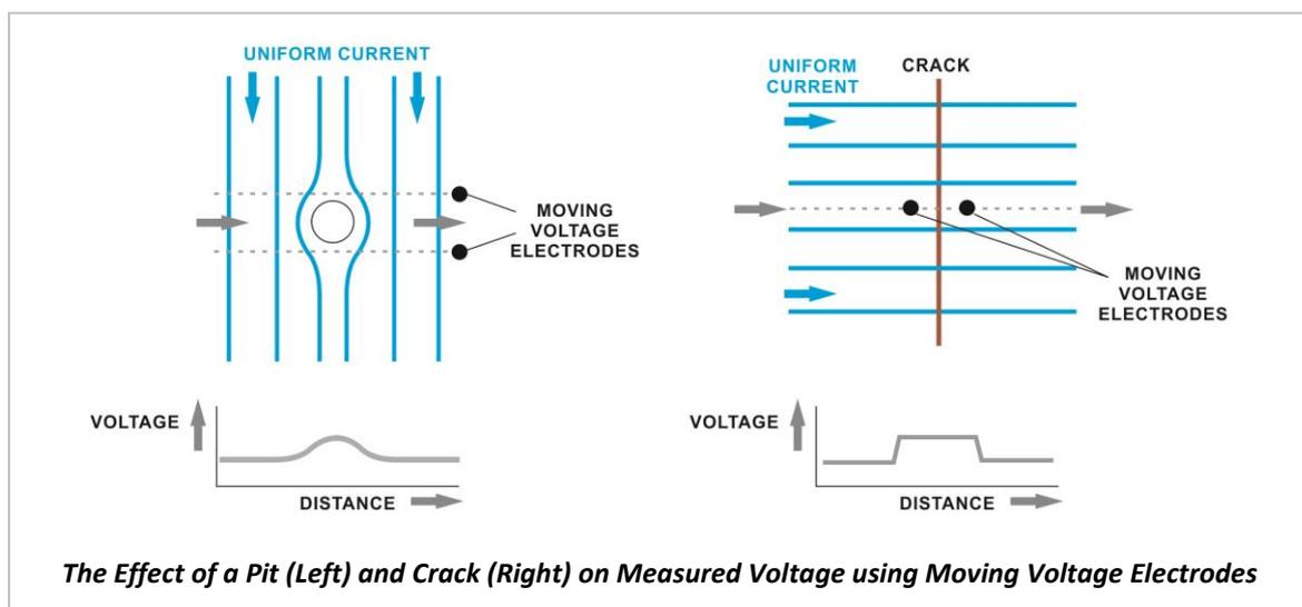
With care, signal 'amplification' might be achieved by locating current electrodes in close proximity to the voltage electrodes and then moving all electrodes over the surface. This produces a high and consistent current density in the vicinity of the voltage electrodes, so amplifying the voltage signals.
