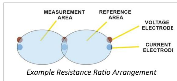
Which approach is used will depend on circumstance: sometimes a practical reference area is not available and so temperature measurement and compensation is needed.
