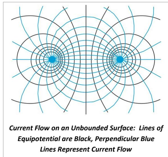
In the case of a pipe, with a point current source and sink positioned along the pipe axis, the current again rapidly spreads out. Assuming an adequate distance between source and sink, the current will quickly and uniformly distribute itself around the pipe circumference.
