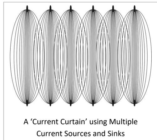
RTL sometimes uses a technique for creating 'uniform' current flow on an unbounded surface using multiple current sources and sinks. This creates what we term a 'curtain' of relatively uniform current flow over a wide surface area, as shown here.
