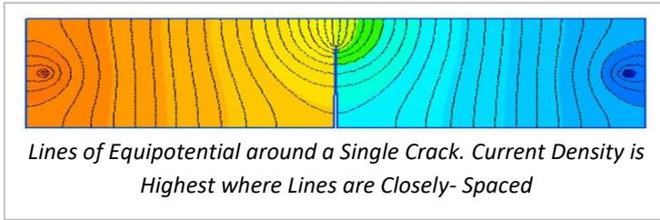
measurement sensitivity: the closer the voltage electrodes are to the growing crack, the greater the observed increases. RTL uses finite element modelling to translate these increases to crack growth.
