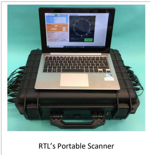
These have been developed for applications where continuous monitoring, using permanently-installed systems, may not be appropriate. An example may be when monitoring at a number of different locations within a large production or process plant.
