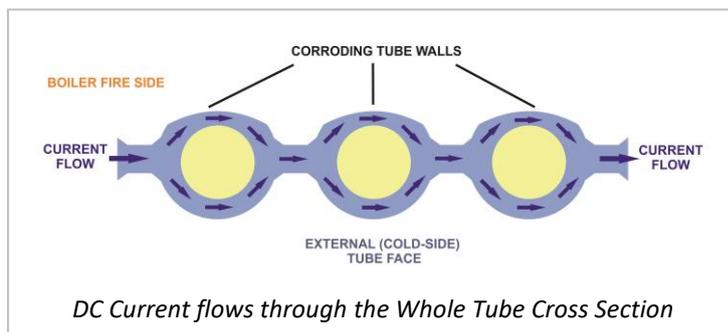
As the fire-side tube wall thins due to corrosion, the measured resistance increases and this is translated into metal loss and corrosion rate. Corrosion is calculated assuming 'uniform' metal loss between adjacent sensor locations.
