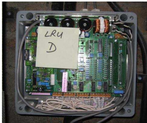
Original LRU Electronics – a Tight Fit meant there was Little Room for Wiring
