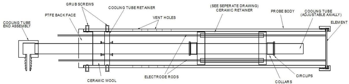
Within the probe bodies a central cooling tube is installed that directs air on to the rear face of the corrosion elements. Measurement electrodes and thermocouples run the entire length of the probe body and emerge at the rear.
