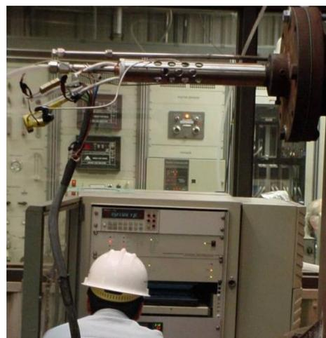
Probe and Monitoring Instrumentation – SRI Combustion Trials
