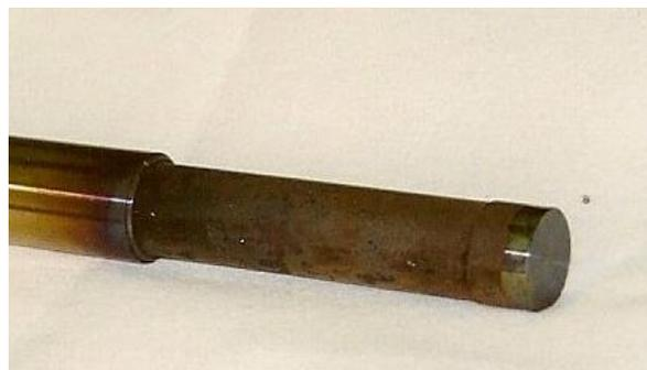
Tubular Corrosion Element
