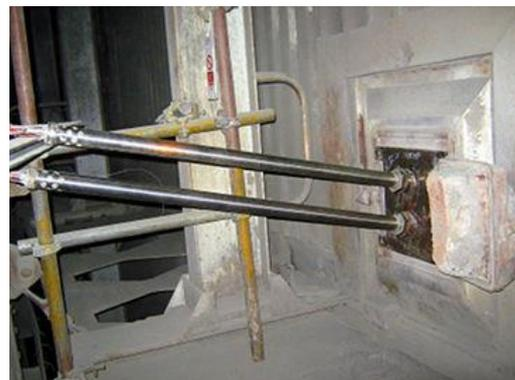
VTER Instrument Cabinet and Probes used for the Biomass Trials
